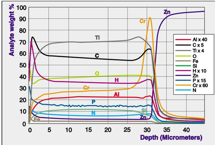
● **Figure 4** Quantitative depth profile analysis of a yellow paint coating on galvanized sheet
