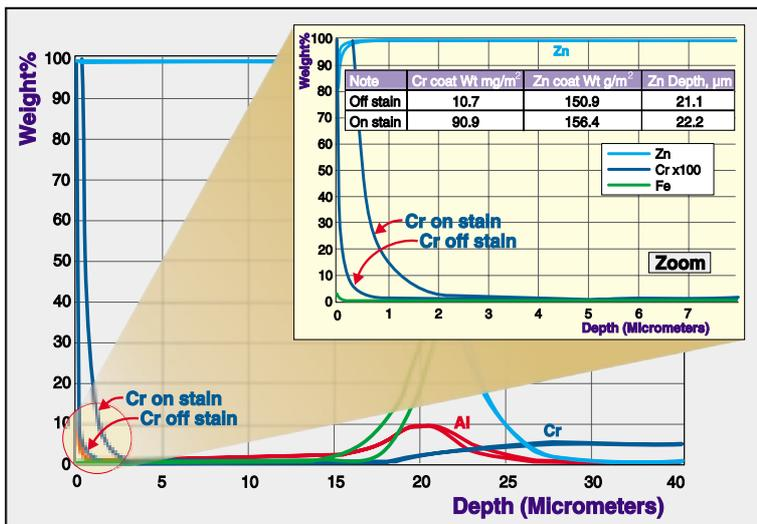
● Figure 3b Detailed profile analysis near the surface of stained and unstained sheets
